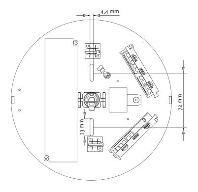
Step 2d/ Drill the holes for canopy and glass component.
