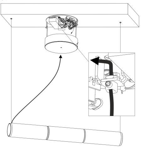
Step 4c/ Connect the cable to the clamps.
