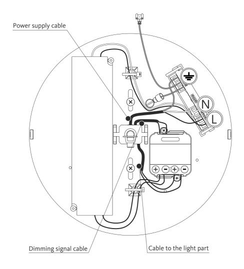
Step 4e/ Secure with a screw. Be careful not to damage the cable.
