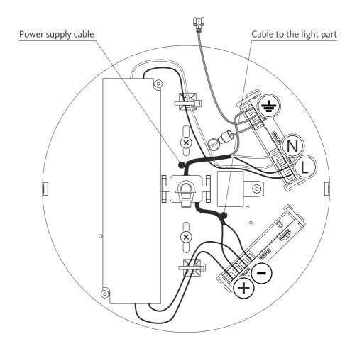
Step 4c.2/ Wiring for DALI dimming
