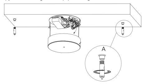
Step 3c/ Hang the glass part. Fix the wire with a reutlinger as shown in the picture.
