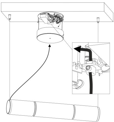
Step 7c/ Connect the cable to the clamps.
