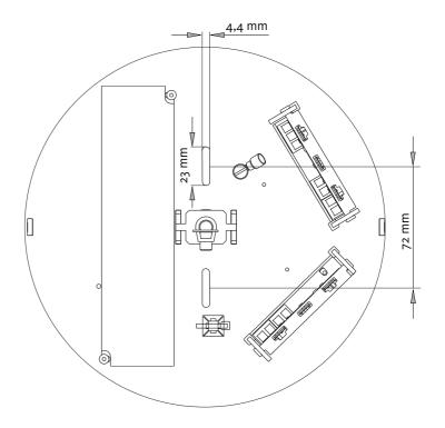
Step 5d/ Cut out the holes for canopy and glass component.
