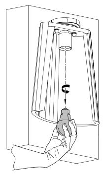
Carry out this step in reverse to fit the new bulb.
